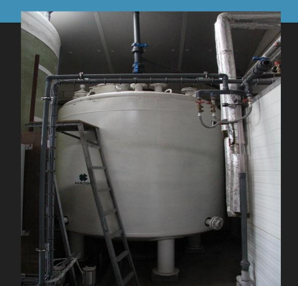
Introduction of bacteria and ferment into the isolated fermentation unit Production of lactic acid
