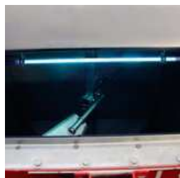
UV Hy Light (Weda) tank disinfection with UV light
